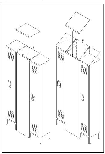
As an alternate method, the 15" wide top filler may be used to cover any gap or front filler width smaller than 15" without trimming the top filler width as shown in the illustration below. Simply use the full width top filler as is and place it into a position straddling the smaller opening between locker tops.
