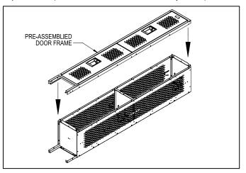
Step 5: Tighten all fasteners, ensuring the locker remains square during the process. If desired, attach optional sloping hood, end bases, or front base (see pages 4 and 5).
