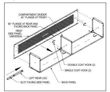
Step 3: Attach a second top shelf, a second bottom shelf, and two additional single coat hooks to a second back panel as in step 1.
