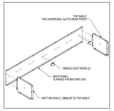
Step 2: Turn the back panel onto its back with the shelves pointing upward. Attach the first side panel, the left rear leg, and the first compartment divider to the assembly from Step 1. Attach two additional single coat hooks to the first side panel, one double coat hook to the bottom of the top shelf, and an additional double coat hook to the bottom of the compartment divider.
