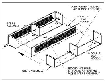
Step 5: Attach a third top shelf, a third bottom shelf, and two additional single coat hooks to a third back panel (as in Steps 1 and 3).
