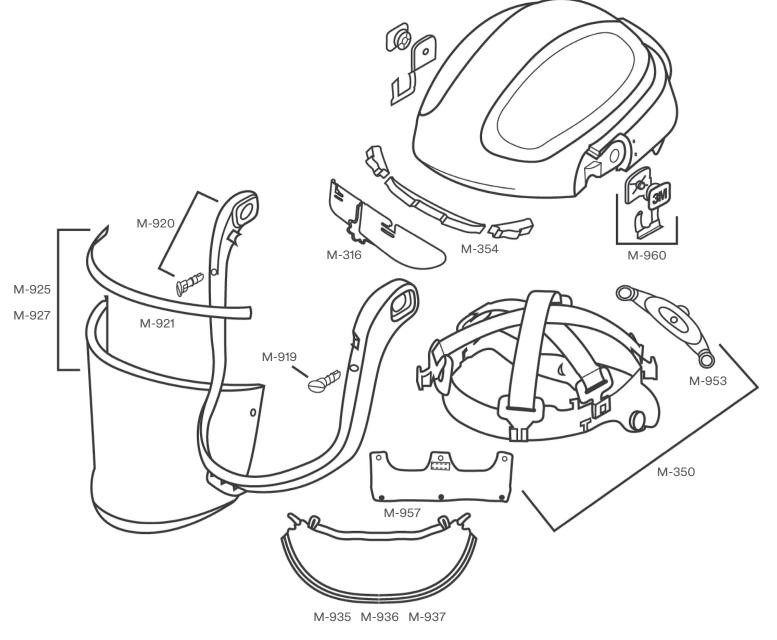
If you discover any signs of wear and/or damage, remove headgear from use and service or replace as appropriate. 3M recommends a maximum life (shelf life plus in use life) of 5 years from the date of manufacture. See the M-Series User Instructions for details on inspection and replacement.
