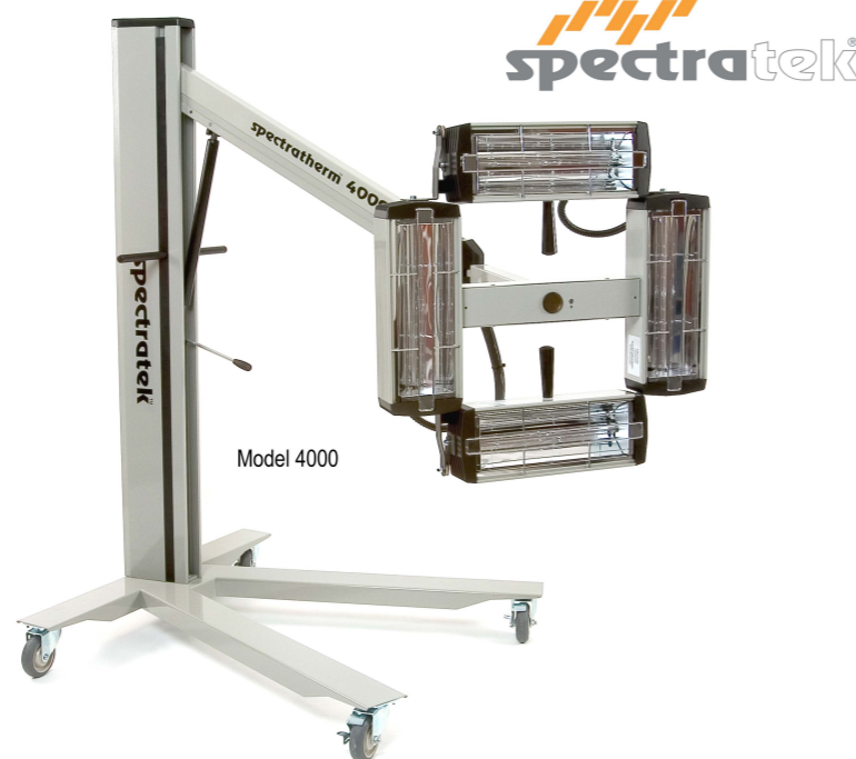
The Spectratek curing system's heating units consist of a tungsten filament, high-temperature halogen-filled quartz lamp, which is encased in an aluminium cassette head with a high precision thermal reflector.
