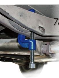
78822 GM HEAVY DUTY TORSION BAR UNLOADING TOOL
