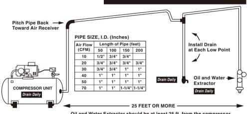
Oil and Water Extractor should be at least 25 ft. from the compressor. Further if possible.
