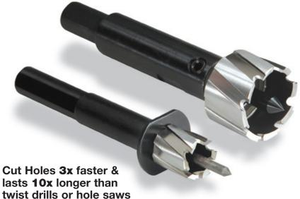
For precision holemaking in sheet metal and frame materials up to 1/2" thick. Blair Rotabroach Annular Cutters make clean, burr-free, round holes with no deforming of stock or damage to the surrounding material. Ideal for sheet metal fabrication or PDR and rustproofing access holes because the snap-in plugs fit perfectly. Custom builders and aftermarket equipment installers can also count on the superior quality holes.
