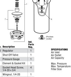
1/2" NPT (female) 14" NPS (male) 120 CFM filter 50 CFM regulator 150 PSI 150°F (65.6°C) 5 micron
