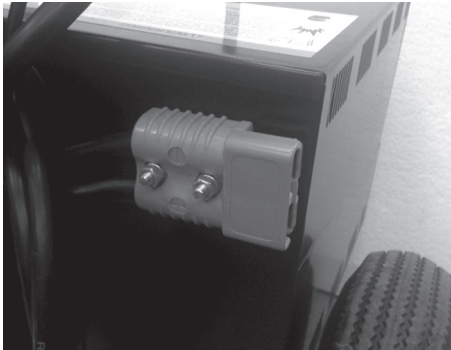
Mounting Gray output power connection.
