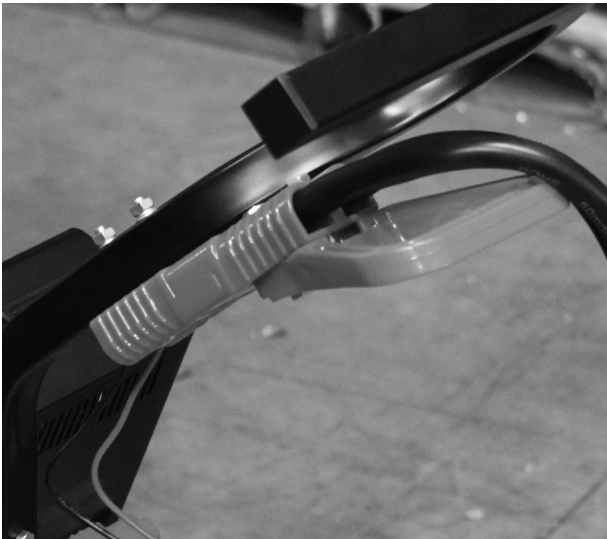
Charging Quick Connect (Red) with Voltage Selection Quick Connect Attached
