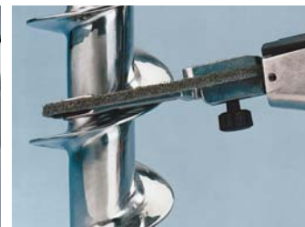
Clean and finish using non-woven nylon belts.
