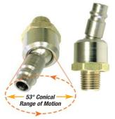
Important: 150 PSI maximum on all models. Do not use on percussion tools or in areas of high mechanical abuse. Note: Do not exceed recommended torque value of 20 ft. lbs.
