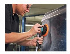
The DynaLocke® quickly strips paint to bare metal when set to rotary mode and converts to random orbital to complete the feather-edging portion of the application.
