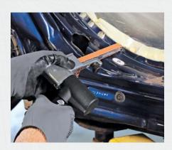
Using a Dynabrade Nitro Series™ NitroFile belt tool body shop technicians can quickly grind through spot welds for a fraction of the cost of using expensive spot weld cutters. Abrasive belt tools also blend welds, grind through seized bolts or even remove seam sealer making them a must-have, versatile tool for any shop.
