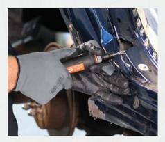
Die Grinders provide a great deal of options for technicians within the body shop. Having a 1/4" collet allows for the use of burrs along with coated and non-woven abrasives in a variety of shapes and sizes.
