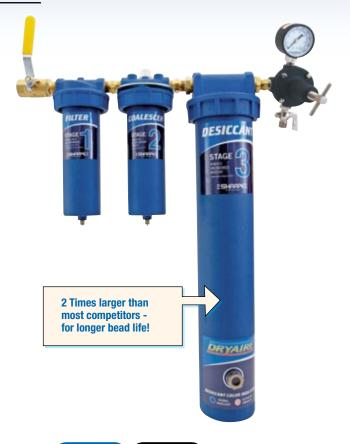
Remove dirt, water, oil and uncondensed moisture from compressed air lines. The Dryaire Desiccant System's 100% indicating silica gel provides maximum moisture absorption. It features easy desiccant change out, regenerate, or replacement (6765-1). This system maintains -40°F dew point while achieving 0% compressed air humidity.
