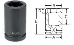
Special 1-1/2" hex deep heavy duty impact socket designed for outer cap nuts on buddstyle truck wheels. The 1-1/2" hex depth is limited to help prevent socket contact with the wheel. The socket is deep style to eliminate contact with the inner cap nut.
