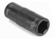
This "flip" style socket features 18.5mm hex on one end and 19.5mm hex on the other. It is designed to remove 19mm lug nuts with missing or distorted caps found on GM or Chrysler vehicles.
