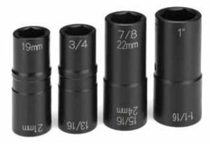
A set of four (4) thin wall "flip" style impact sockets that have two different hex sizes in each socket. Sockets are designed for auto and light truck wheel fasteners. Use with 1/2" drive extended shank impact tools or regular shank impact tools with an extension.
