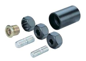
This kit removes inner cap nuts on budd wheels when the square head of the nut has broken off. Also included are rib nuts to remove 5/8" and 3/4" spoke wheel studs. Simply drive the rib nut over the broken cap nut or wheel stud and remove with an impact wrench.
