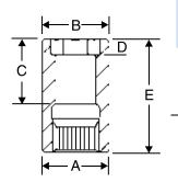
Special 1-1/2" hex deep heavy duty impact socket designed for outer cap nuts on budd-style truck wheels. The 1-1/2" hex depth is limited to help prevent socket contact with the wheel. The socket is deep style to eliminate contact with the inner cap nut.
