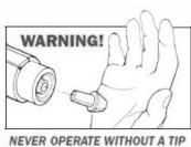
Select Tip: Insert tip into electrode bore making sure of positive contact. Select Puller type: Chose 2.2 or 2.6 Uni-stud.
