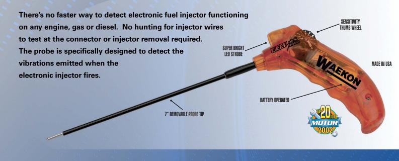
Simply press the 7" long probe tip against the injector body, adjust the sensitivity using the thumb-wheel and the bright LED strobe will flash each time the injector opens and closes. The strobe allows the you to determine if the injector is firing consistently, misfiring or not firing at all.
