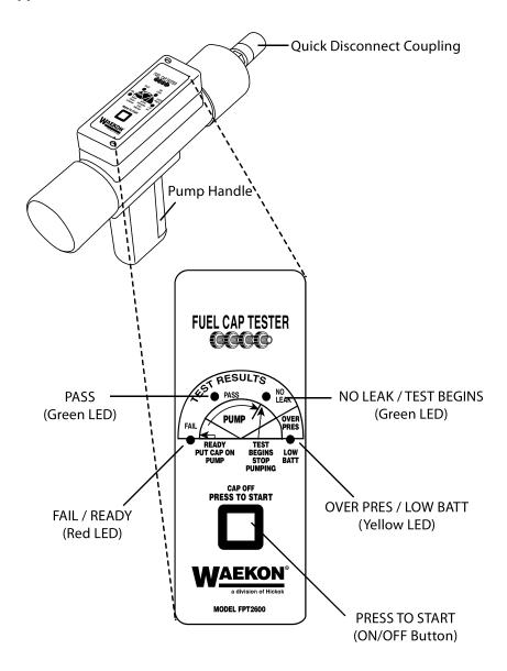
**PRESS TO START** (ON/OFF Button)—Pressing this button turns the power on and off.
