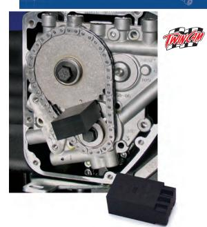
**CAM/CRANK SPROCKET LOCK TOOL** This precision tool allows the technician to lock the camshaft and crankshaft sprockets to properly remove, replace and torque the sprocket bolts. This tool is made from non-marring Delrin. *For more details see No.1285-IS instructions*.
