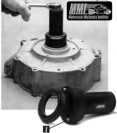
SPROCKET SHAFT BEARING NUT WRENCH
