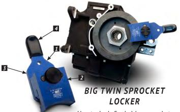
Use to lock final drive sprocket, for removing and installing sprocket nut. Use with JIMS<sub>®</sub> tool No.94660-37A. For more details see No.2260-IS instructions.
