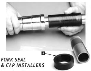
Use to install fork seals, dust seals, and chrome caps. Lightly grease to keep from scratching fork tubes. For more details see No.2044-IS instructions.
