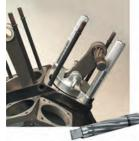
use with their designed lead in taper at the start of each ream. Use JIMS° No.1284 Rod Clamp tool. For more details see No.1726-IS instructions.
