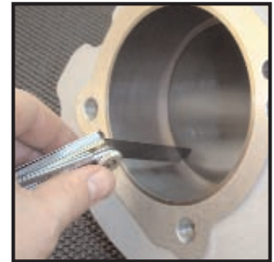
Fig.17 - Feeler gauge gap
