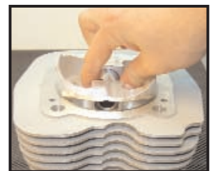
Fig.19 - Press ring down
