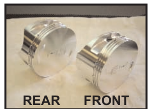
Fig.33 Note piston notch
