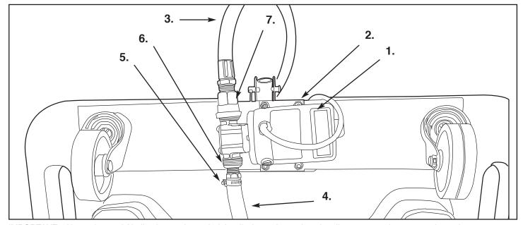
IMPORTANT - Always keep 1/2' ball valve on the end of the discharge hose closed until you are ready to empty the tank.
