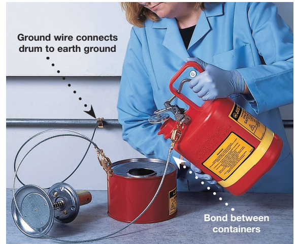
Bond dispensing can to receiving container, then ground receiving container to a water pipe or ground strip.
