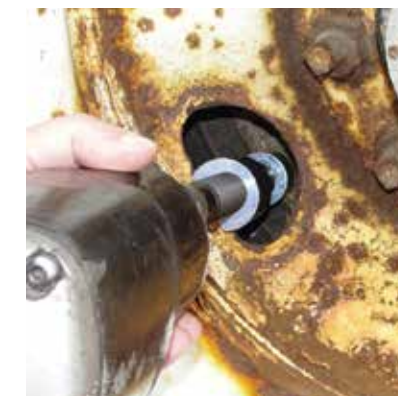
Pusher is ball bearing-driven for near-zero turning resistance and is heat treated for long-lasting strength and durability
