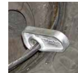
Newest Bead Holder - Made From Aluminum
