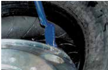
BENT END For mounting and demounting bottom bead
