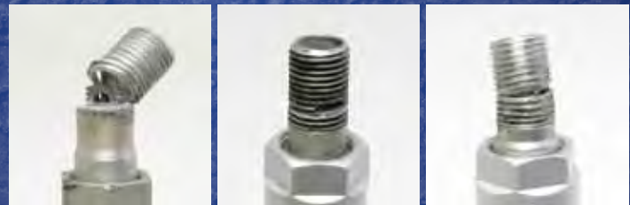
Galvanic corrosion causes TPMS failures.
