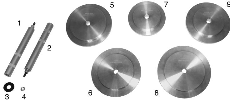
The set includes 5 drivers. The driver is designed to hold the seals to make installation easier. Includes handle extension for driving bearing races and seals on hubs with deep brake drums without removing the drums. For applications that do not need the length of the two-piece handle use only the handle with the solid end. Do not hammer on the tapped end of the handle extension. Use the included hardened washer between the driver and handle to protect the aluminum driver.
