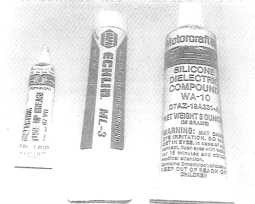
Figure 7.8. Some of the safe lubricants you can use in place of the Dow-Corning 111 grease. Oddball lubricants may damage rubber brake parts.
