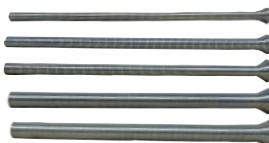
Economical and effective tools for bending soft copper or aluminum tubing without kinks. Special nickel plated, spring steel is flared on one end for quick tube insertion. Each tool bends one size.
