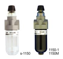
A visible drip type lubricator with an external adjustment screw. Unit is designed for low air flow applications where space is a consideration. Requires approximately 1 CFM of air flow to deliver oil. Bypass system allows full air flow with minimum pressure drop. Assures proper air/oil mixture over full operating range
