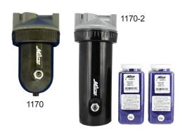
Delivers extremely dry compressed air as low as -30°F dew point without using electricity or refrigerant. Easy to monitor, when color changes in the sight glass from dark blue to pink, then it is time to change or dry the desiccant. To dry desiccant, remove from unit, bake at 275°F for 3 hours. To prolong the life of the unit, a 40 micron pre-filter, and .03 coalescing filter should precede dryer. Initial supply of desiccant is included
