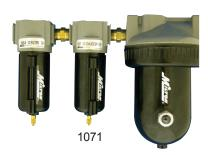
Not only dries the compressed air, but also removes dirt and oil. Each factory assembled system consists of the components listed below. Both filters are equipped with Milton® automatic overnight drains that will drain when the system drops below 5 PSI. Initial supply of desiccant is included
