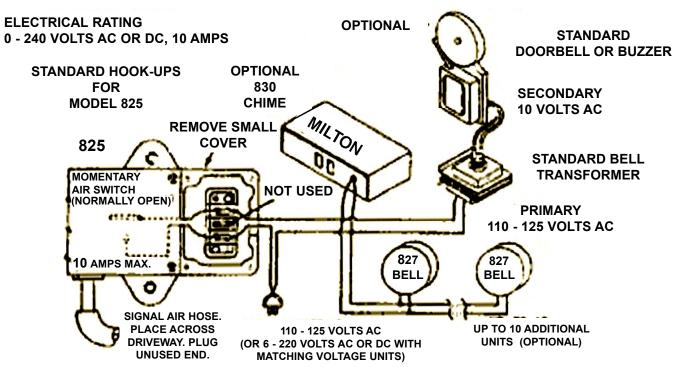
This is a pictorial wiring diagram to suggest various hook-up options and to show a typical circuit path. Any installation must be properly terminated and insulated and must conform to all applicable codes. Consult a qualified electrician.
