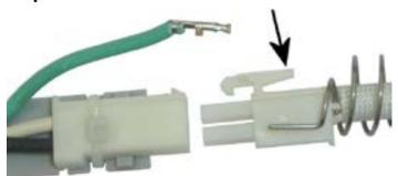
Push the locking lever to unhook the ceramic heater core and unplug the ceramic heater core from the power lines.
