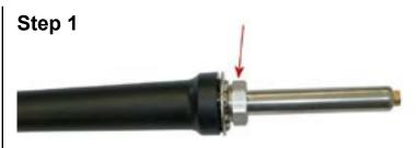
Remove the large nut at the base of the barrel and slide the barrel off of the assembly.
