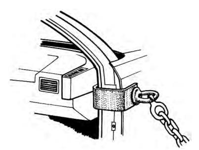
Use this new hook from Mo-Clamp to pull front hinge pillars, center pillars posts, rear hinge sections or any location where you need a broad, thin pulling surface.
