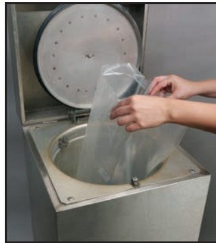
Inserting bag into distillation tank.
