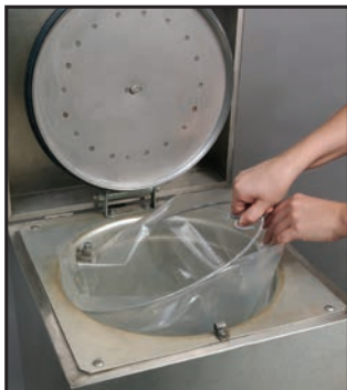
Securing bag with retaining ring.
