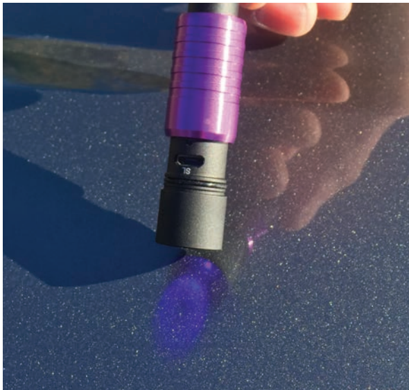
Expose UV primer or clearcoat to UV light at close range for 20 seconds
