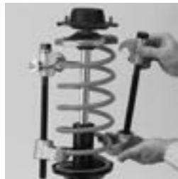
1. Attach clamps to spring
