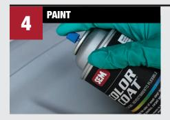
Apply Bumper Coater flexible coating, Color Coat flexible coating, Sure-Coat flexible coating, Trim Black, or Trim Black Ultra trim paint.
