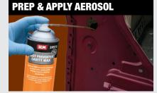
Clean surface with SEM Solve or XXX Universal Surface Cleaner where applicable. Remove cap from Rust Preventer Cavity Wax, attach straw or Rust Preventer Aero Wand. Apply 1-2 coats.
