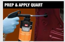
Clean surface with SEM Solve or XXX Universal Surface Cleaner where applicable. Shake bottle of Rust Preventer Cavity Wax for 1 minute. Spray 1-2 coats at 35-45 psi.
