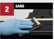
Sand primed surface with P180 grit sandpaper Blow off & tack clean. Re-clean with *SEM* Solve or XXX Universal Surface Cleaner. Wipe clean in one direction with clean, lint-free cloth.
