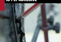
Apply 3/8" - 1/2" bead of **Dual-Mix™ Multi-Purpose Panel Adhesive or Dual-Mix Weld-Bond Adhesive** to both surfaces. Use enough material to completely fill the joint when parts are clamped. Tool with a spreader or acid brush. Cover all exposed bare metal.
