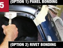
Clamp panel into place. Do not over clamp. Wipe away excess material.
