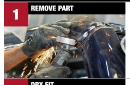
Remove spot welds with spot weld cutter. Remove rivets by drilling or grinding. Remove damaged panel and straighten bent flanges with a hammer and dolly.
