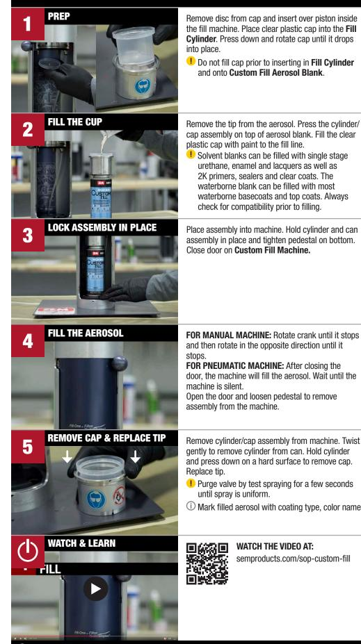
Remove disc from cap and insert over piston inside the fill machine. Place clear plastic cap into the Fill Cylinder. Press down and rotate cap until it drops
