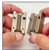
Pins ensure accurate alignment of dies
